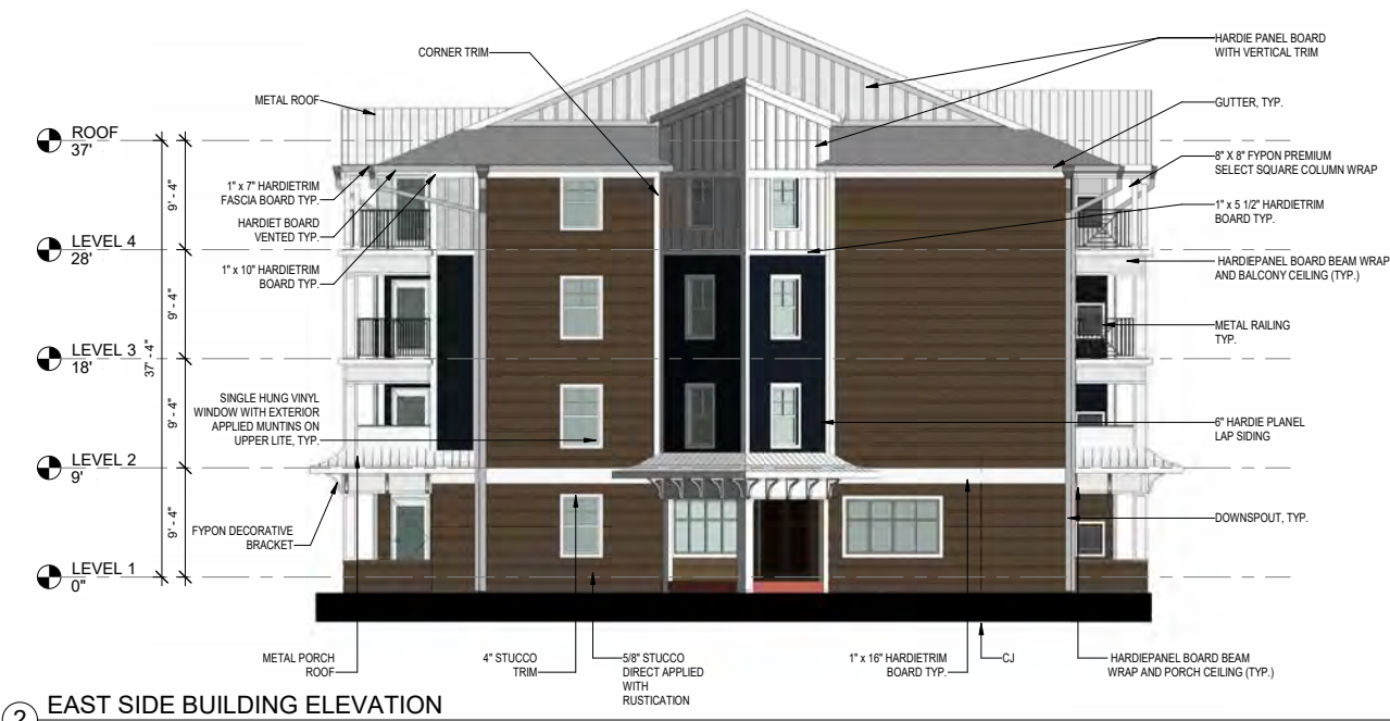
2 EAST SIDE BUILDING ELEVATION
